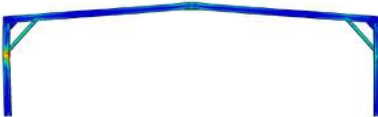
Fig. S.6 NLFEA shell model of 22 m span frame: displacement and buckling under applied vertical load at ambient temperature
