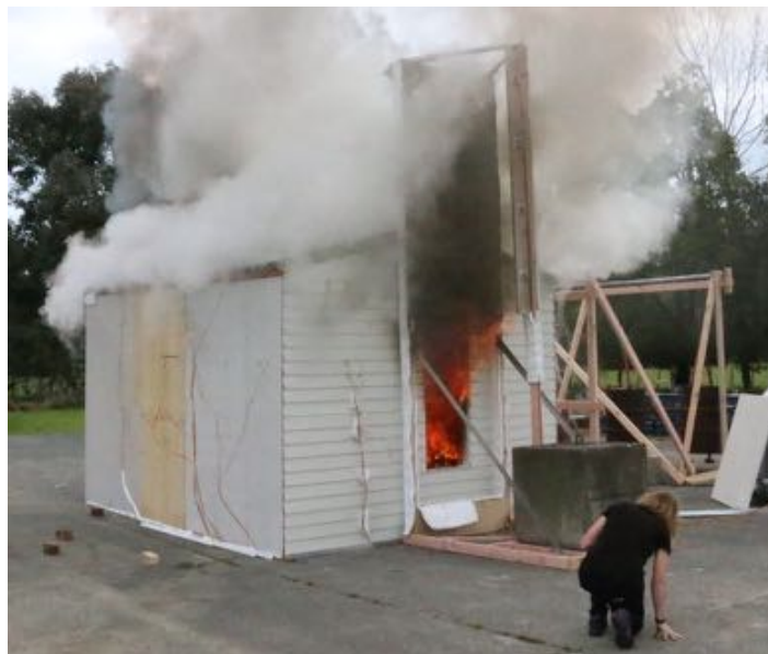
Approx. time of ceiling failure, t \approx 13 min
