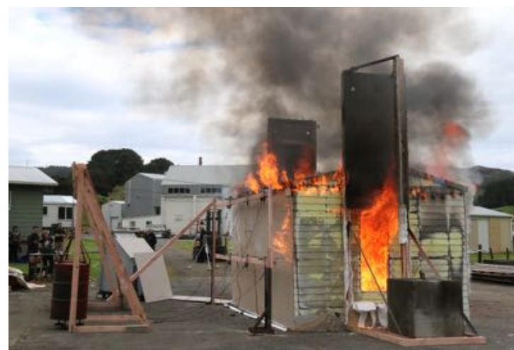
Fire-rated wall failed under lateral load & roof partially collapsed, photo at t \approx 30 min
