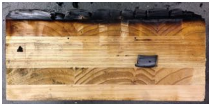
Typical char profile of sample before removing the char layer
