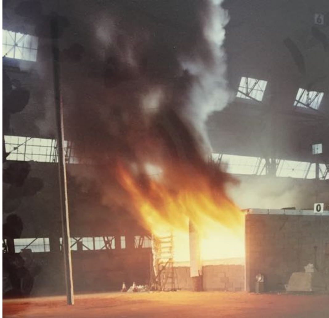
One of the fully developed fires in the tests, 50% ventilation
