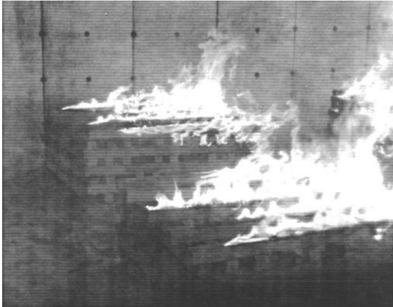
Example of spontaneous ignition of top of cribs due to radiation from hot gas layer in one of the tests
