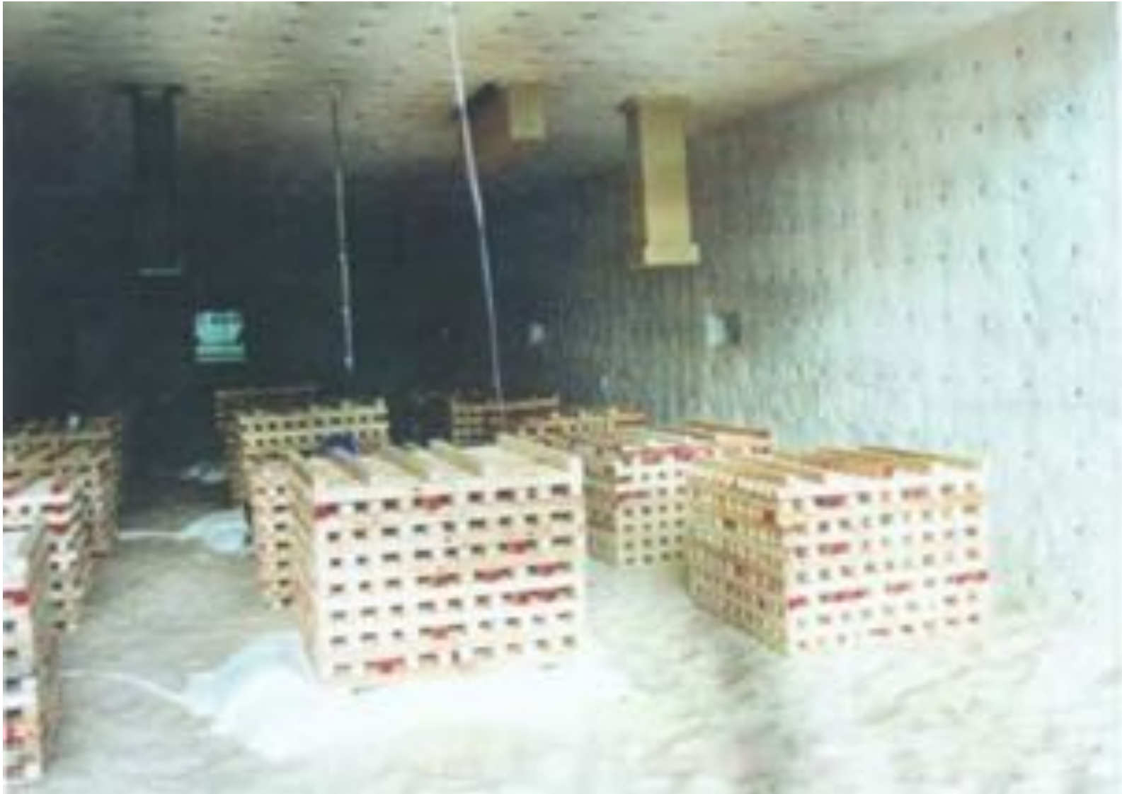
Crib construction in progress (40 kg/m 2 floor area shown here)
