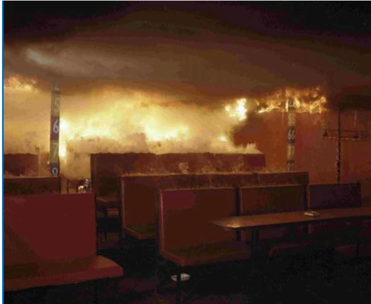
Seconds before flashover - BRE simulation of Stardust Disco disaster fire. Fire about to 'jump' across tops of bench seats resulting from hot gas layer radiation. Example of autoignition.
