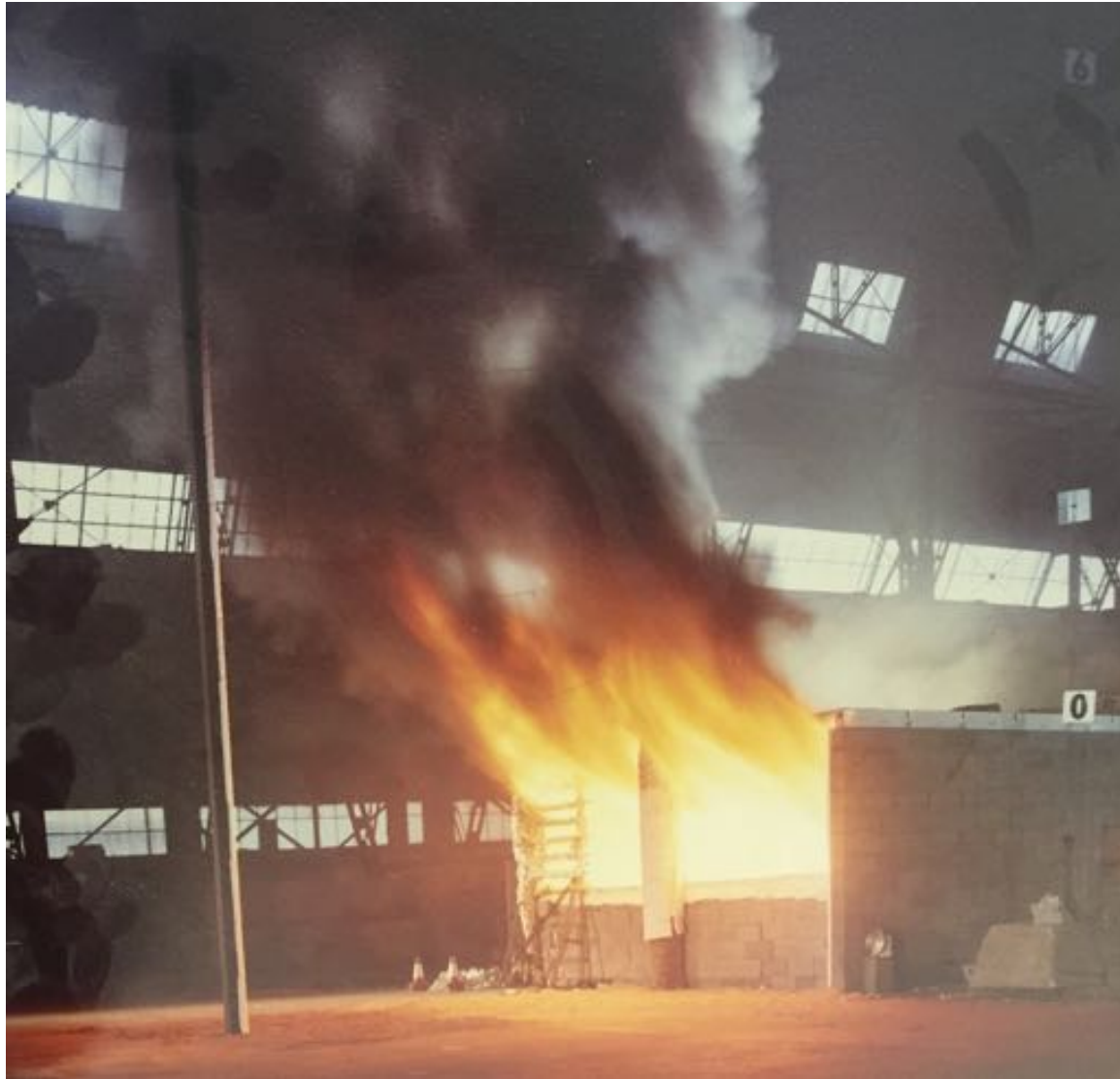
Fully developed fire with 50% ventilation
