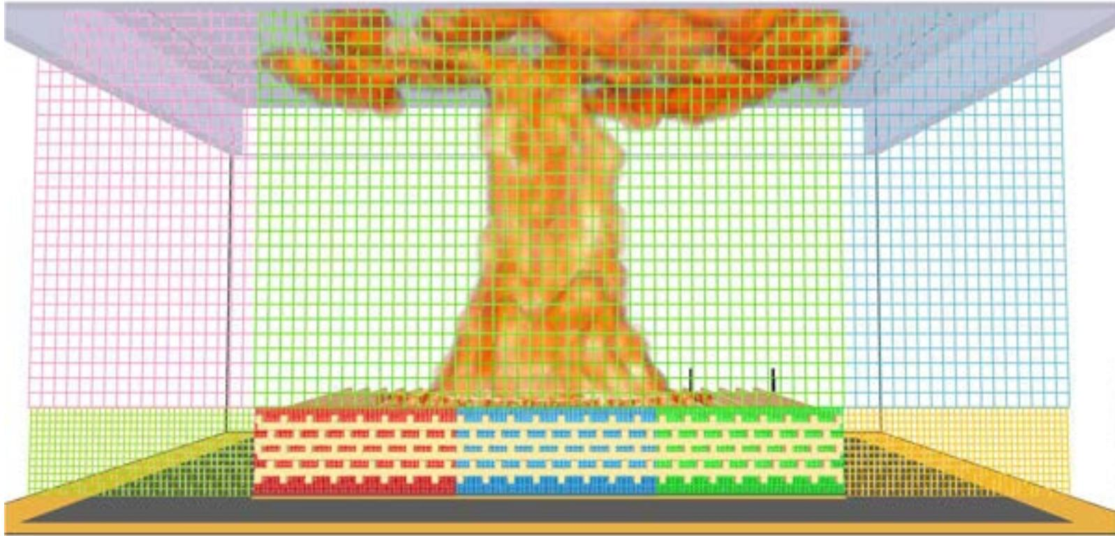
Grid cell resolution of the model:  $1.5 \times 1.5 \times 1.75$  cm per cell for wood sticks in porous crib structure,  $6 \times 6 \times 7$  cm and  $3 \times 3 \times 3.5$  cm cell size in gas phase, total no. cells  $\sim 1.3$  million.
