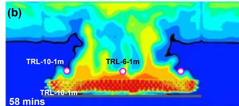
Gas phase temperature contour of the compartment 'slice' at specific time, (a) TRL-1/4/9 'slice' at 32 mins, (b) TRL-2/6/10 'slice' at 58 mins.
