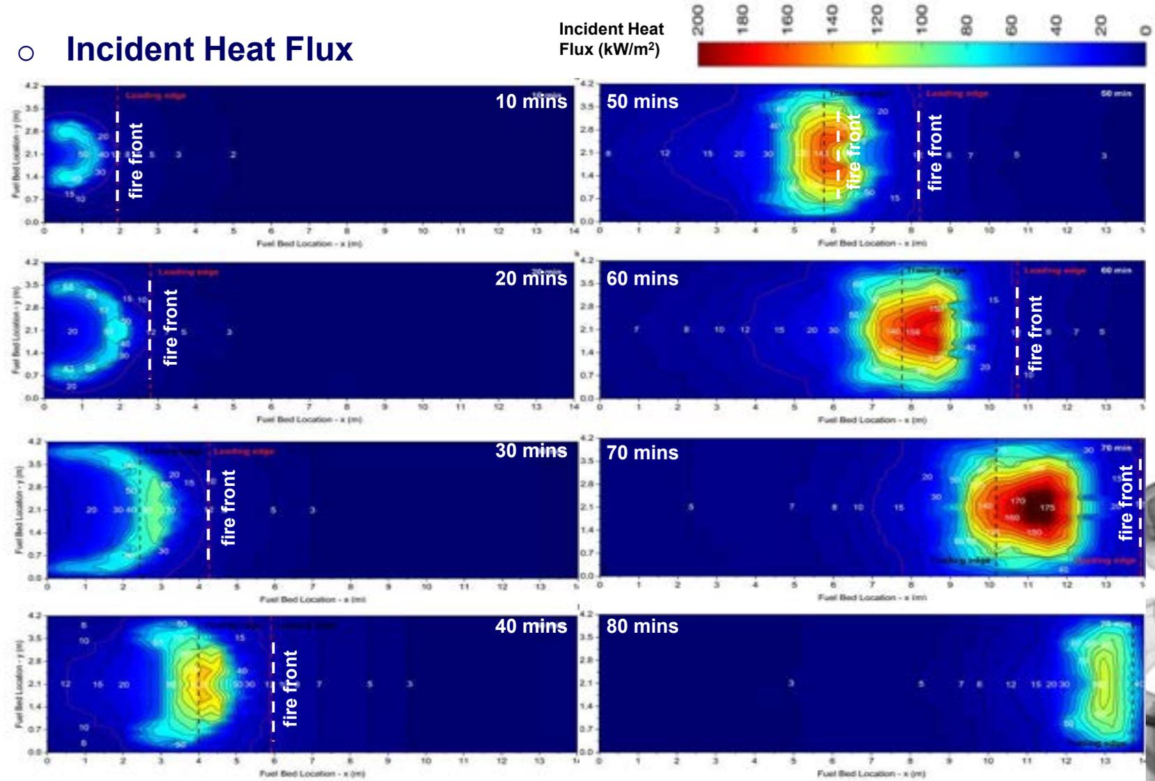
Incident heat flux on the top layer of wood sticks with 10 mins intervals
