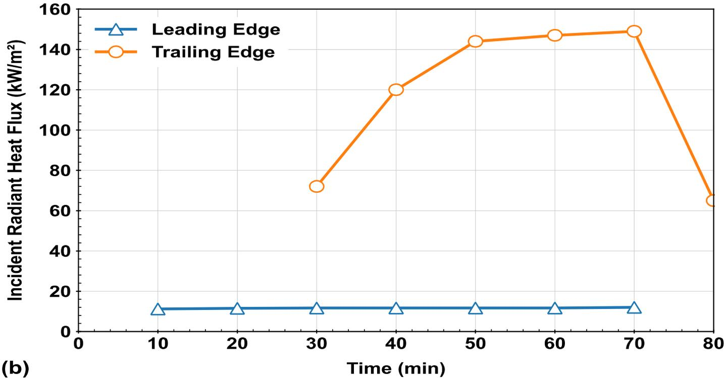
(b) Comparison on incident heat fluxes from thin skin calorimeters (TSC) at fuel bed top level centreline along fire trajectory (TSCF-3 failed during test data acquisition after 30 mins).
