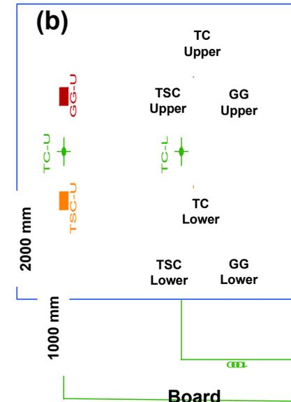
Location of the heat fluxes instrumentations, (a) plan view, TSCF-1 to TSCF-5 were thin skin calorimeters (TSC) on top of the fuel bed level, (b) board in elevation view, instrumented TSCs, Gordon Gauges (GG), and thermocouples (TC).
