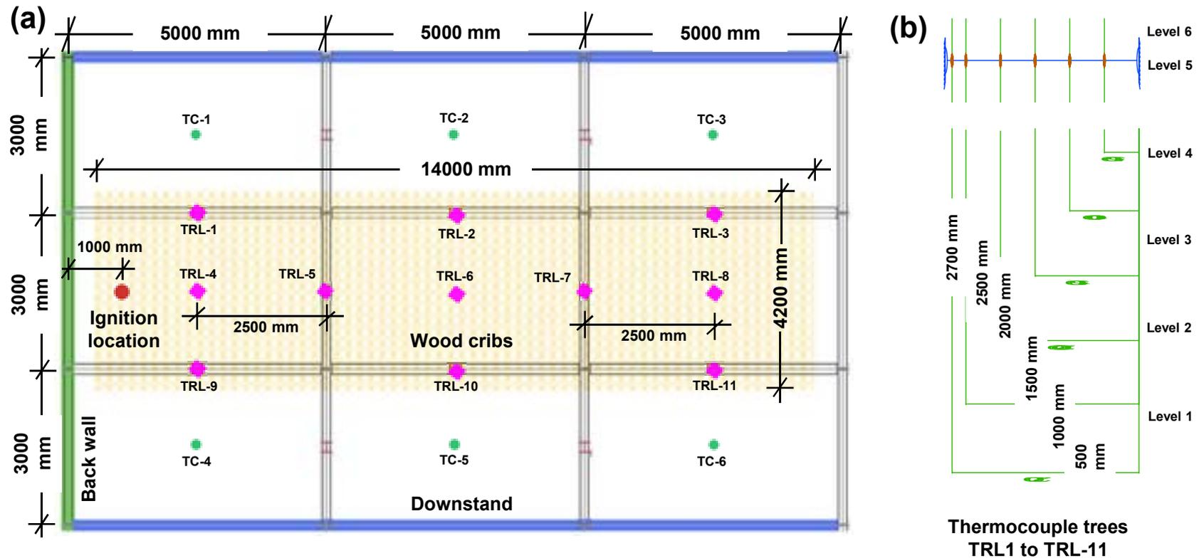
Location of the thermocouples for measuring gas phase temperatures, (a) plan view, TC-1 to TC-6 were thermocouples 200 mm below ceiling, (b) elevation view, TRL-1 to TRL-11 were thermocouple trees above the wood cribs.
