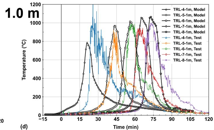
Comparison of thermocouple temperatures at compartment centreline along fire trajectory, TRL-4 to TRL-8, (a) ceiling level (note: TRL-5-2.7m failed during test data acquisition), (b) 2 m from floor level, (c) 1.5 m from the floor level, and (d) 1 m from the floor level (i.e., 0.265 m from the fuel bed top level).
