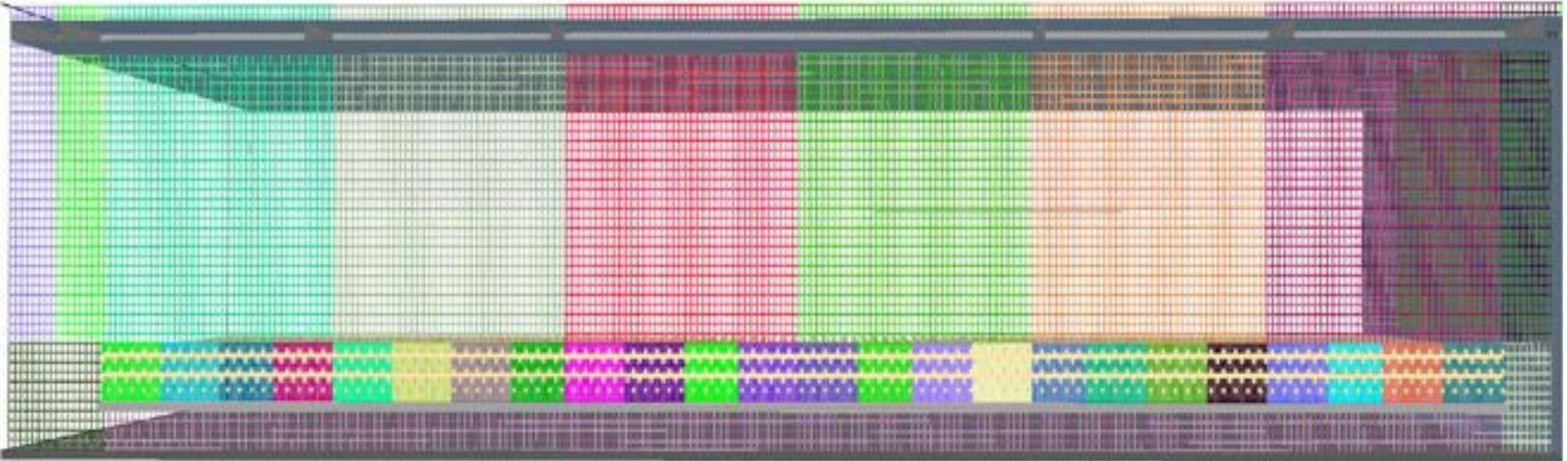
Grid cell resolution of the model:  $15 \times 15 \times 17.5$  mm per cell for the wood sticks at solid phase,  $60 \times 60 \times 70$  mm and  $30 \times 30 \times 35$  mm cell size at the gas phase, total no. cells  $\sim 8.3$  million, with 125 meshes.
