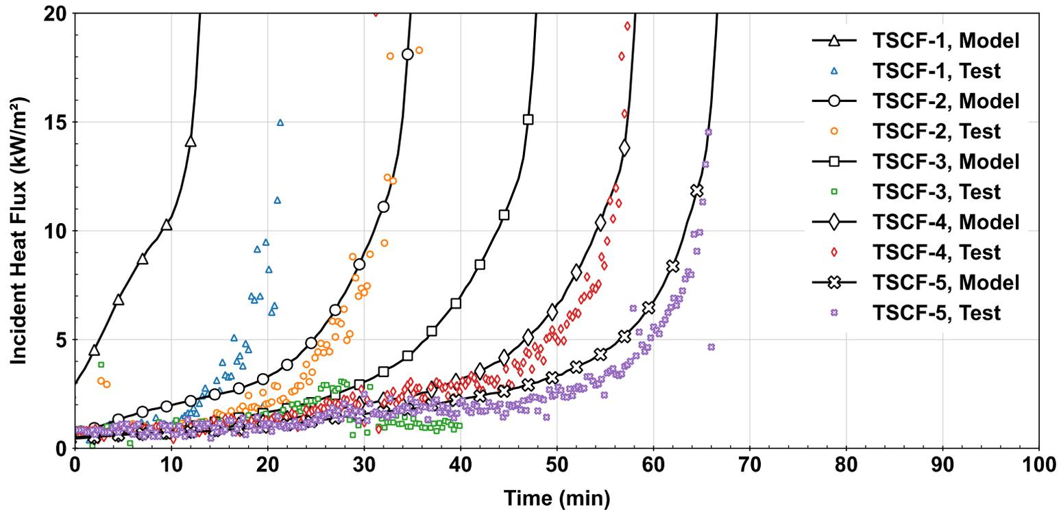
Comparison on incident heat fluxes from thin skin calorimeters (TSC) at fuel bed top level centreline along fire trajectory (TSCF-3 failed during test data acquisition after 30 mins).
