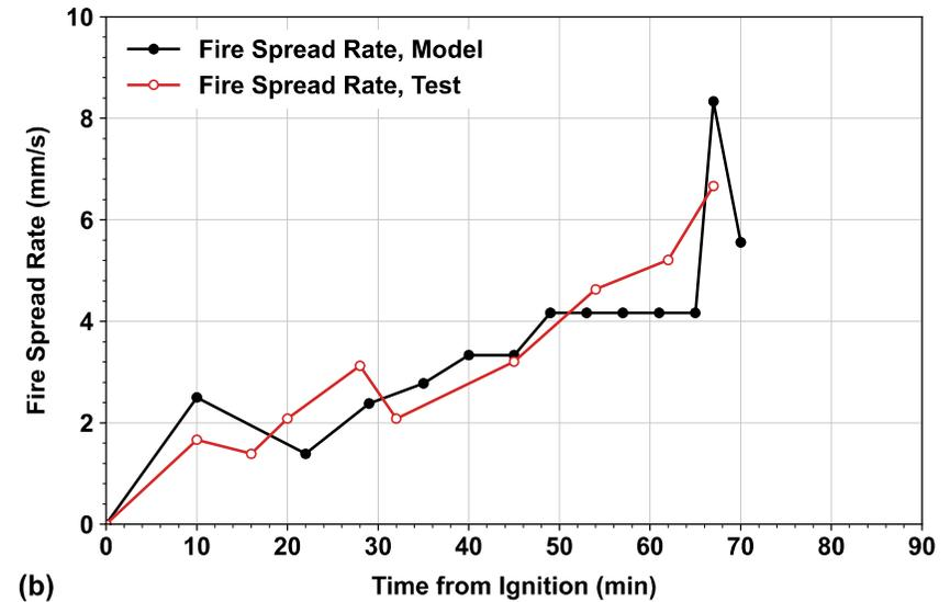
Comparison between the test and the model at compartment centreline along fire trajectory, (a) Fire spread distance & burn-away, and (b) Fire spread rate.
