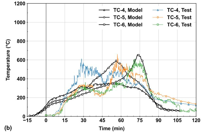
Comparison of the thermocouple temperatures, 200 mm from the ceiling level at side bays, (a) TC-1 to TC-3, and (b) TC-4 to TC-6.
