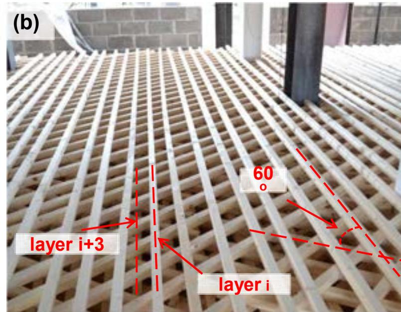
Wood sticks arrangement, (b) Wood sticks orientation shifted  $60^\circ$  every layer, and for every three layers shifted horizontally for half of the wood stick pitch, same arrangement as the LB7 test from Gamba et al. [xx].
