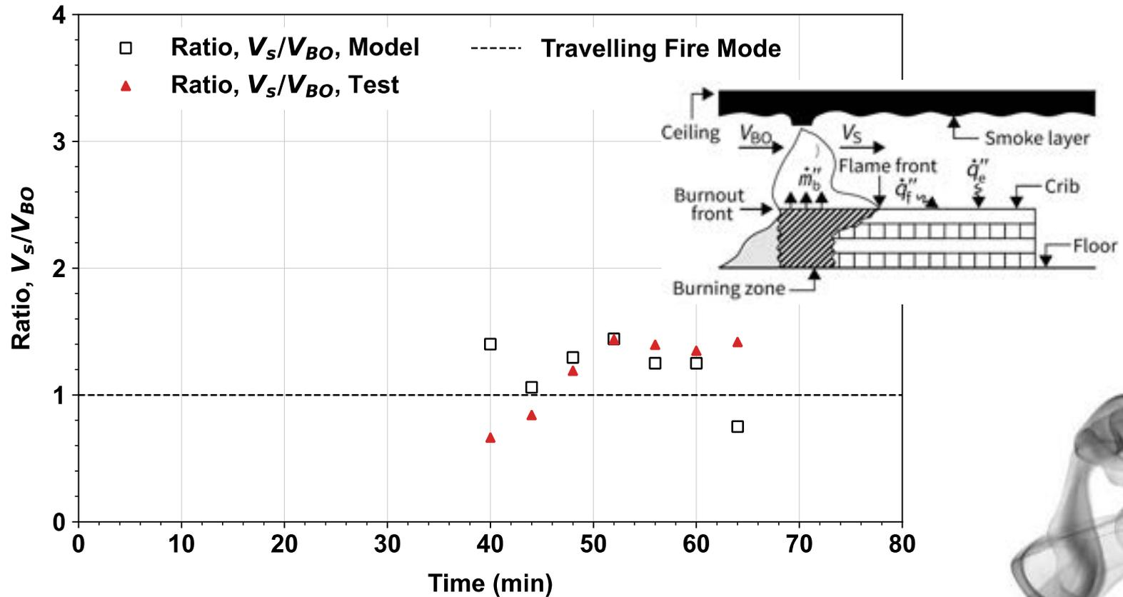
Comparison on fire mode parameter,  $V_s/V_{BO}$ : velocity of the flame spread front to velocity of the flame burnout front.
