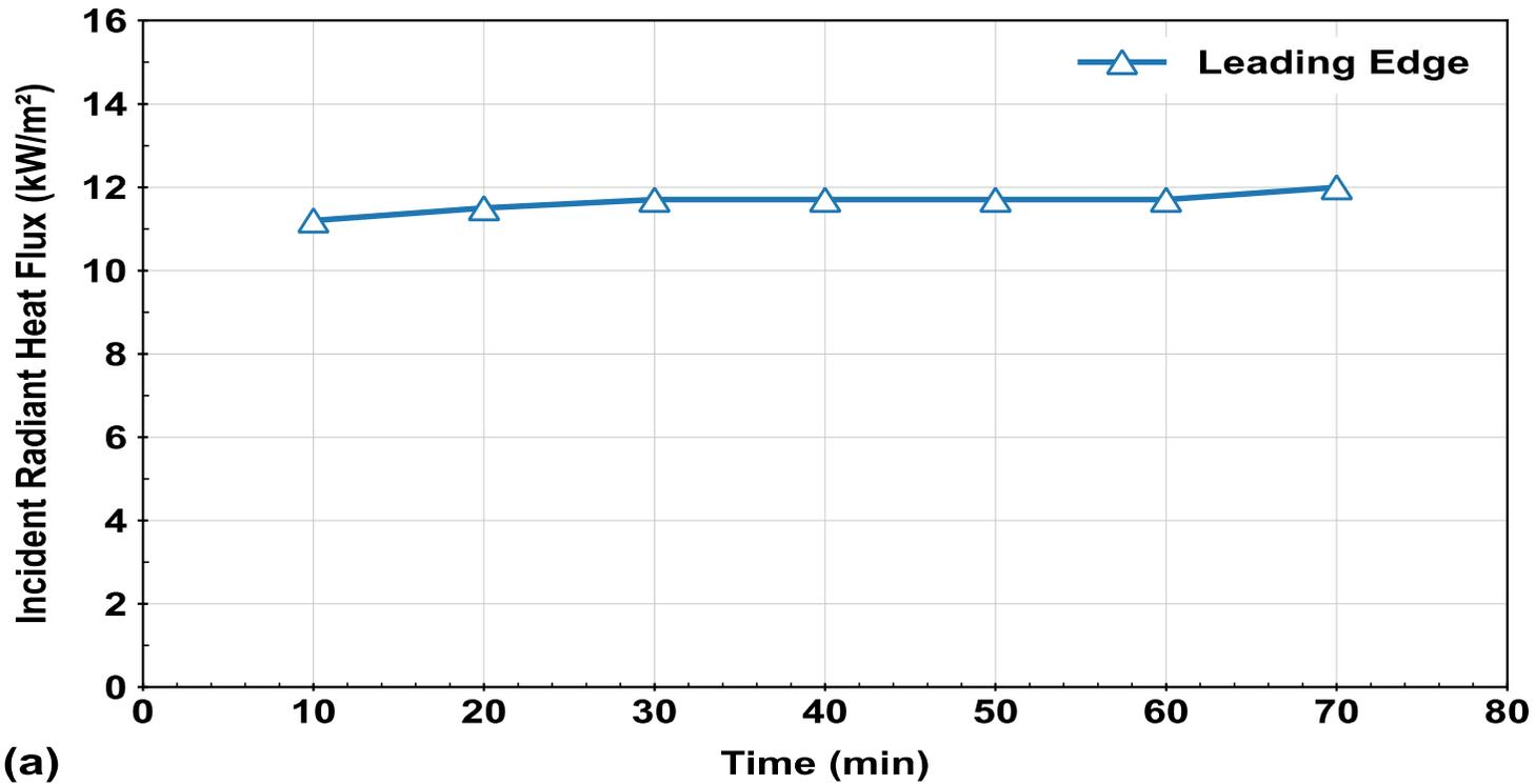
(a) Comparison on incident heat fluxes from thin skin calorimeters (TSC) at fuel bed top level centreline along fire trajectory (TSCF-3 failed during test data acquisition after 30 mins).
