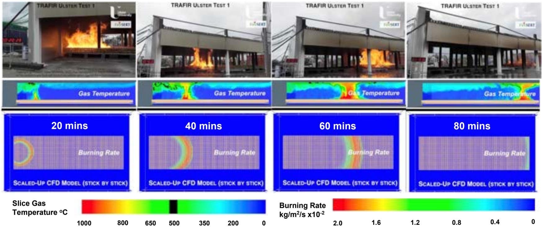
Scaled-up CFD model predicted fire spread comparison with the test, at 20, 40, 60 and 80 mins
