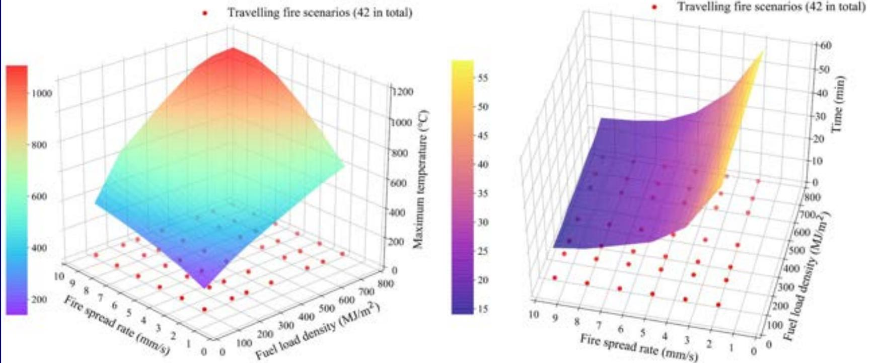
Various combinations of different fire spread rates (ranging from 2 mm/s to 9.5 mm/s) and fuel load densities (ranging from 100 MJ/m<sup>2</sup> to 780 MJ/m<sup>2</sup>) with 42 travelling fire scenarios, marked with red dots as sampling points, with (a). maximum steel beam bottom flange temperatures at location 00; (b). time to reach the peak temperature of the steel beam bottom flange at location 00.
