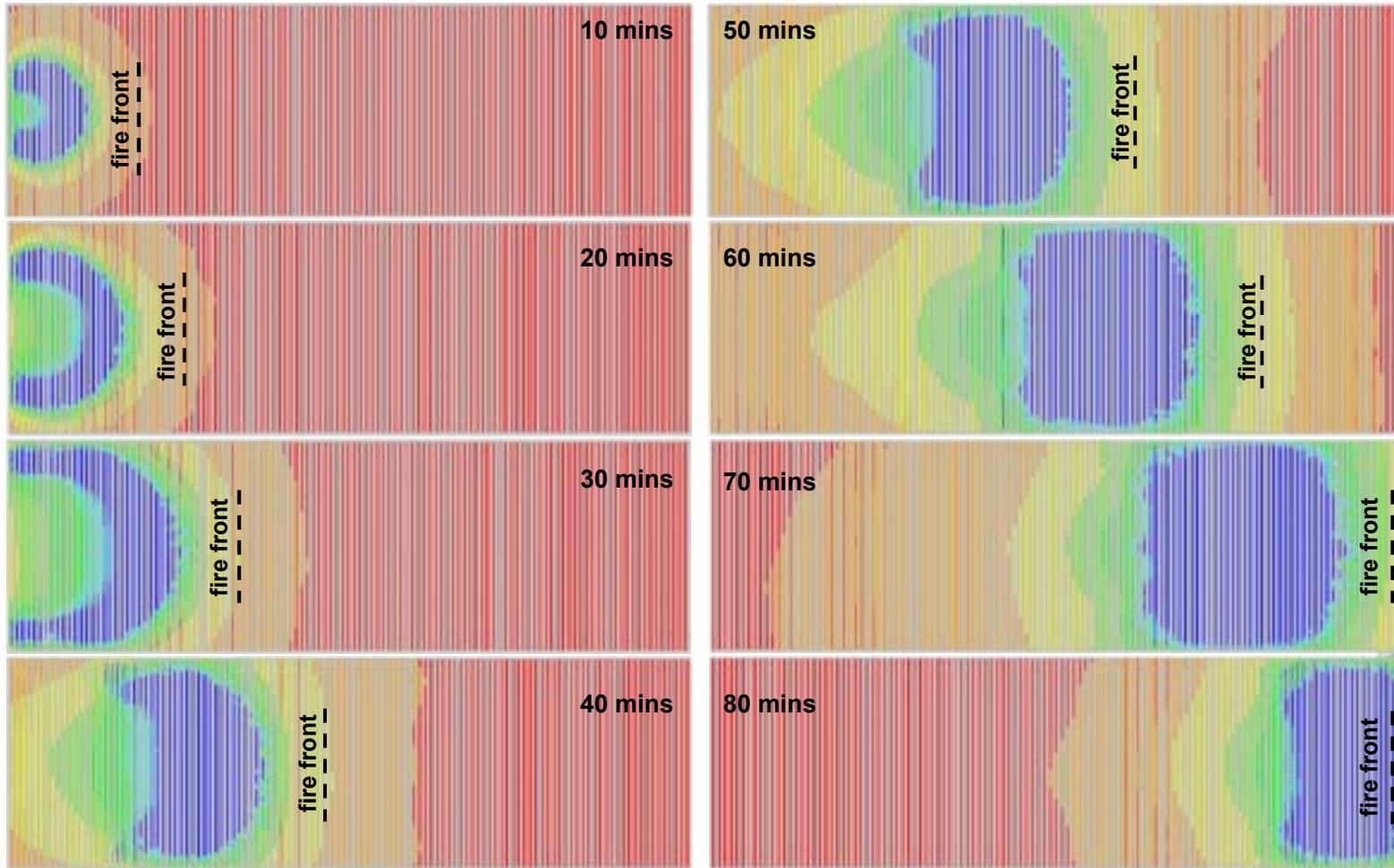
Incident heat flux on the top layer of wood sticks with 10 mins intervals
