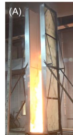
Agarwal, G., Wang, Y., & Dorofeev, S. (2020). Fire performance evaluation of cladding wall assemblies using the 16-ft high parallel panel test method of ANSI/FM 4880. Fire and Materials , April, 1–15.
