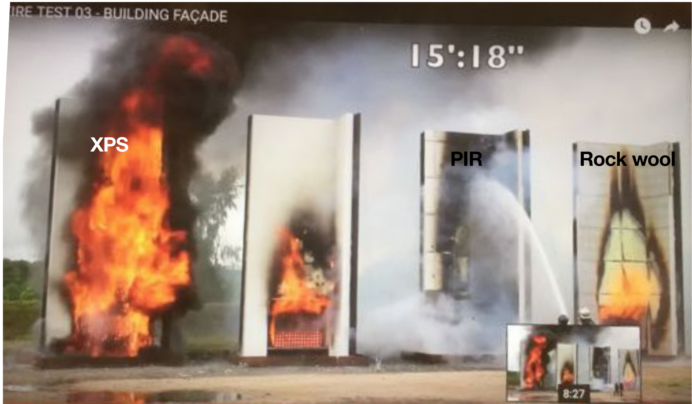
Extreme left, XPS foam flaming over entire height
