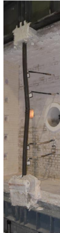
SHS 80×80×3-2500 specimen Failure mode.
