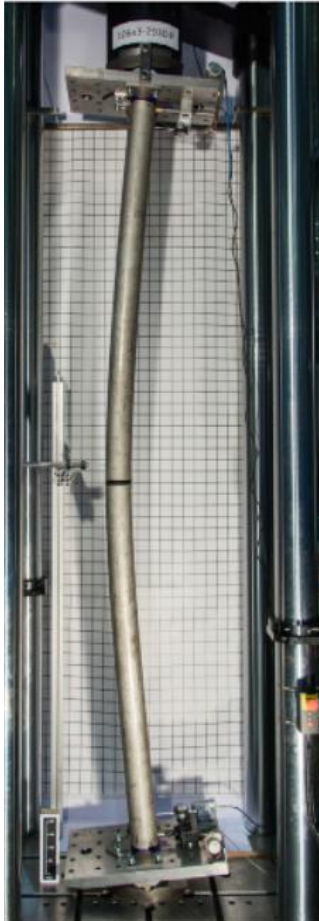
CHS test and FE model column failure mode.
