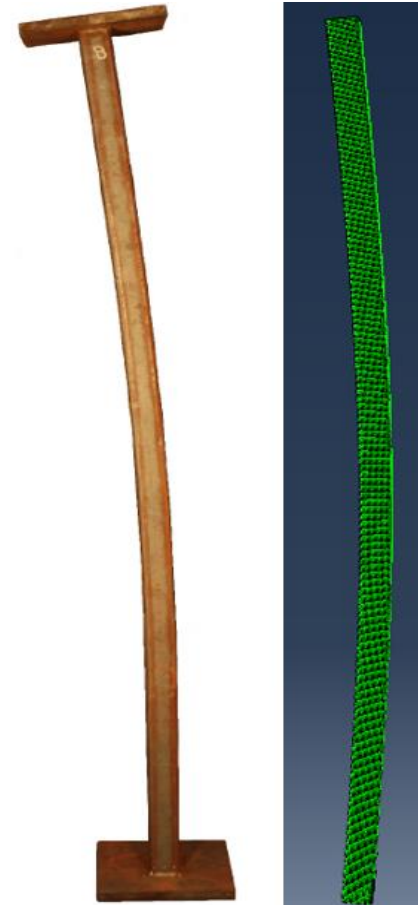
Test and FE failure mode for elevated S355 steel beam-column specimen RHS 120×60×4-(7).
