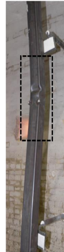
SHS 80×80×3-2500 specimen Failure mode.
