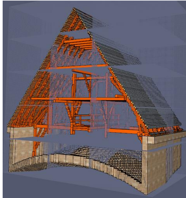
Notre Dame FDS model: 9 x 14 x 15 meter (choir) – meshing
