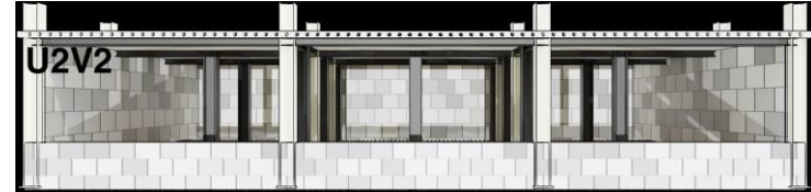
Fig 11 Parametric study on opening factors and areas extended from Ulster TRAFIR Tests 1 and 2 (U1, U2)
