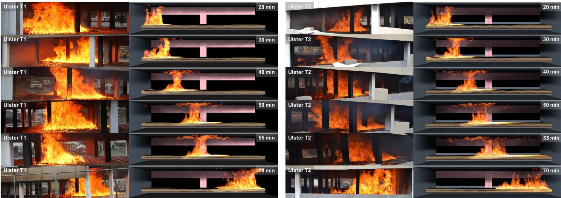
(a) Fig 21 Comparisons of fire spread between test and model at compartment centreline along fire trajectory every 10 mins: (b) a) Ulster TRAFIR test 1 (well ventilated IOF=1.6 m -0.5 ) b) Ulster TRAFIR test 2 (transitional IOF=8.1 m -0.5 )
