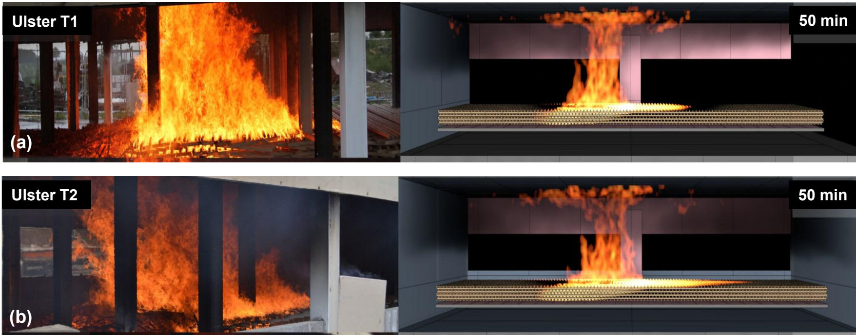
Fig 22 Comparisons of fire spread between test and model at Ulster compartment centreline at 50 mins: a) test 1 b) test 2
