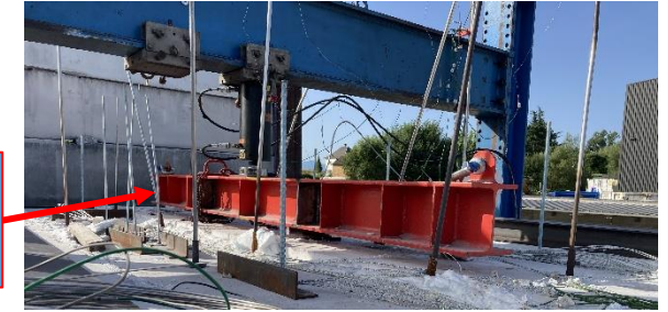
Hydraulic loading on the steel beam
