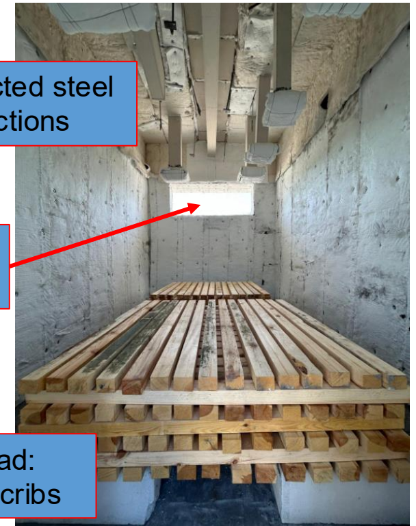
Wooden cribs and protected steel elements before the test 13
